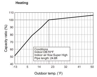
Heating operation ambient temperature range is -31°F~75°F
