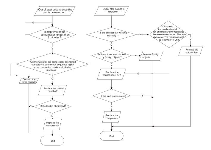
(6)Overload and air exhaust malfunction diagnosis (following AP1 for outdoor unit control board) Mainly detect:
