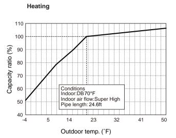
Heating operation ambient temperature range is -13°F~75°F
