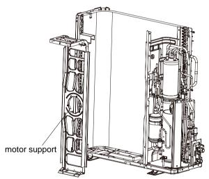
10.Remove 4-way valve assy and electronic expansion valve assy
